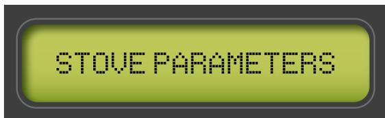
Press SET to open and modify the main stove parameters such as pellet load, flue gas extraction speed, ambient air fan and ambient temperature correction. Using the TEMP+ and TEMP- keys it is possible to change the stove setting percentages to correct its operation based on the pellets used. Then press SET to confirm the modified parameter and save it in the memory. Use the PROG+ and PROG- keys to scroll the parameters.
