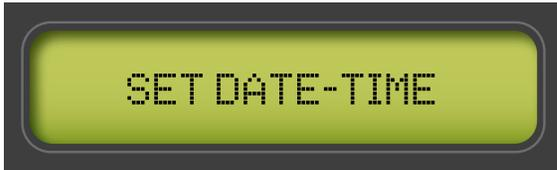
Press SET to open the incorporated calendar setting menu. The day of the week can be changed from Monday to Sunday, as well as the time and date. To switch between the variables, use the PROG+ and PROG- keys, and to change the values, use the TEMP+ and TEMP- keys. To confirm the changes and exit, press the SET key.
